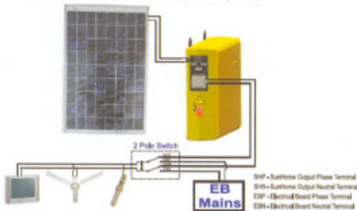
SunHome system connected through existing wiring
